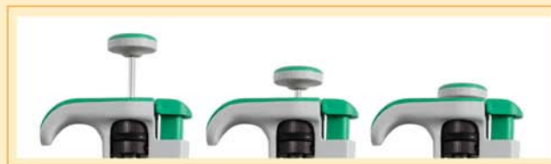
Figure 2.13. Plunger positions of micropipets. From left to right, plunger at rest, at soft stop, and at hard stop.
