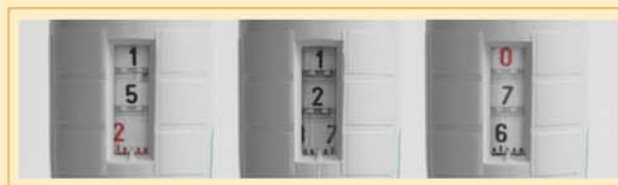
Figure 2.12. Dial readout from adjustable-volume micropipets. From left to right, 2–20 µl, 20–200 µl, and 200–1,000 µl micropipets reading 15.16 µl, 127.4 µl, and 758 µl, respectively.
