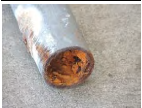
Photo #48: Deteriorating water pipe
